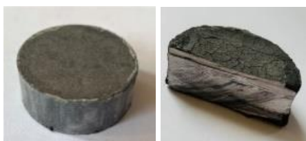
Figure 1. Appearance of the initial pressing (left), sample after reaction synthesis (right)
