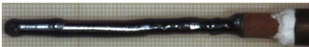
Figure 1. TTB lanthanum rod obtained by the floating zone method
